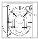
3. Remove the 4 protective screws and the rubber bush with the respective spacer, situated on the rear of the appliance (see also the installation leaflet).
